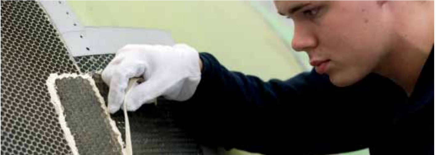
One common cause of nacelle repairs is the disbonding of honeycomb structures as a result of corrosion.
